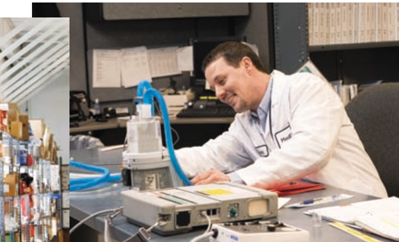
Home Care Services technician Tony Dahl performs function and maintenance checks on a portable ventilator.
