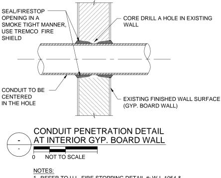
1. REFER TO U.L. FIRE STOPPING DETAIL #: W-L-1054 & W-L-1252 FOR FIRE STOPPING REQUIREMENTS.
