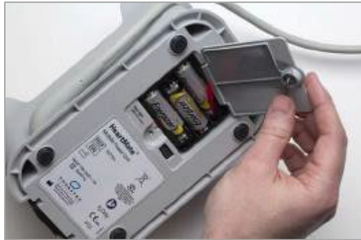
Figure 2 – Remove the battery compartment cover
