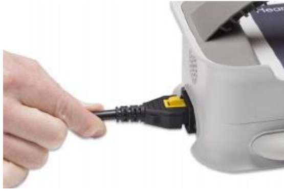
Figure 5 - pull back to ensure a secure connection
