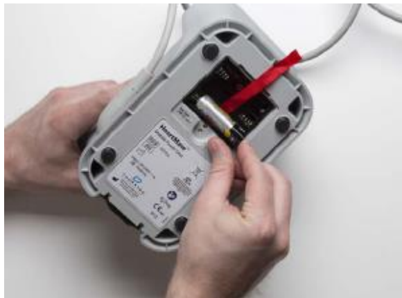
Figure 3 - replace the batteries
