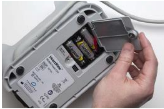
Figure 2 - remove the battery compartment cover
